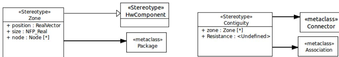
Figure 2. Extension of the profile to enable the description of Zones and Contiguities in composite diagrams.
